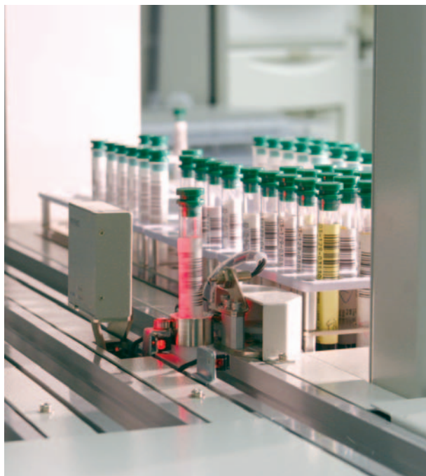
Figure 6: Laser based barcode-driven sorting for clinical immunology testing.
