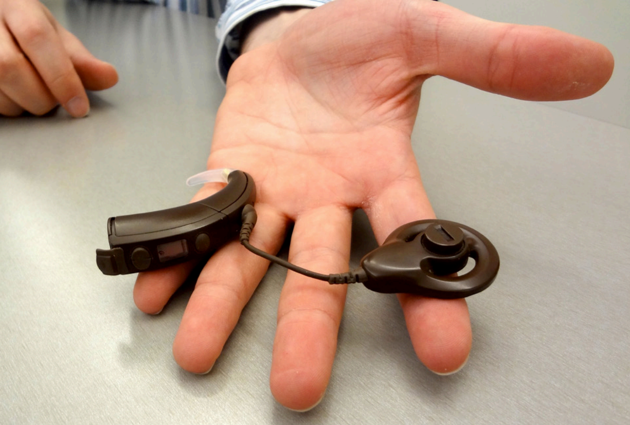
The external Nucleus Freedom Cochlear Implant Jordan wears on his ear, which communicates with an implanted receiver.
