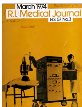
Figure 2. March 1974 Single probe rectilinear scanner illustrated an introduction to nuclear medicine and imaging modalities in use.
